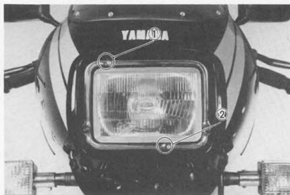
1. Horizontal adjusting screw 2. Vertical adjusting screw
