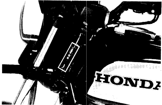
The vehicle identification number (VIN) is on the steering head left side.
