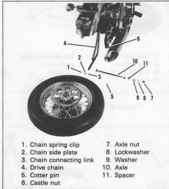
Figure 2-12. Removing Rear Wheel (1973 and Later)
