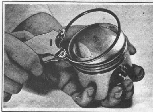
Figure 3-15. Assembling Rings with Ring Expander
