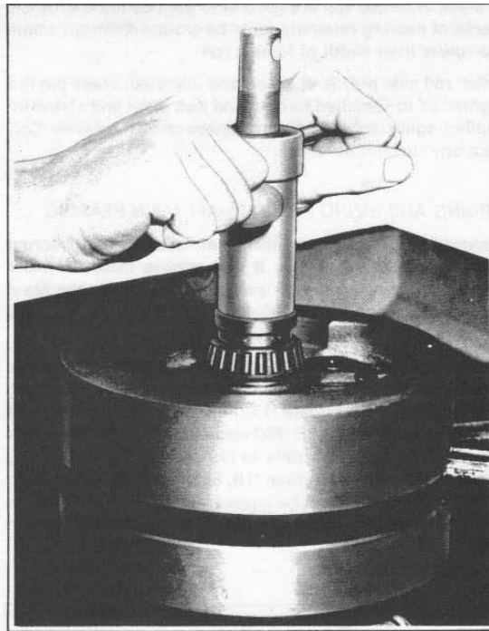
Figure 3-49. Pressing Bearing on Sprocket Shaft
