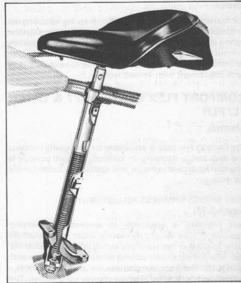
Figure 2-70. Cutaway of Seat Post Springing
