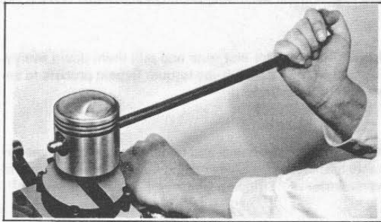
Figure 3-18. Straightening Connecting Rod
