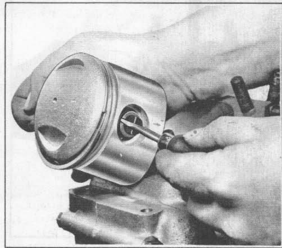
Figure 3-9. Removing Piston Pin Lock Ring (1972 and Earlier)
