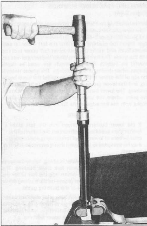
Figure 2-44. Installing Fork Slider Bushing
