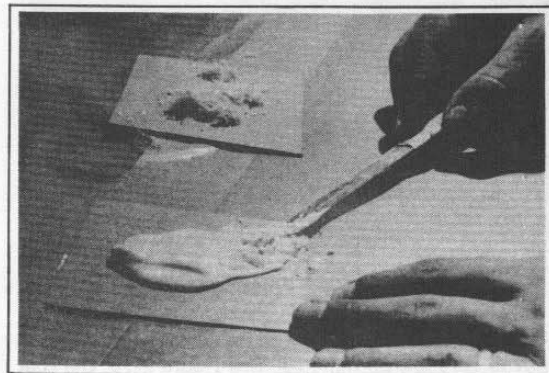
Figure 2-75. Mixing Gel Coat Glass Fibers
