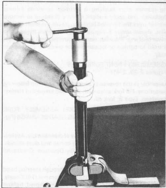
Figure 2-43. Removing Fork Slider Bushing
