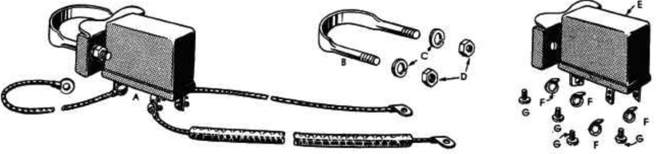
FIGURE 06 - 6—GENERATOR FIELD SWITCHES
